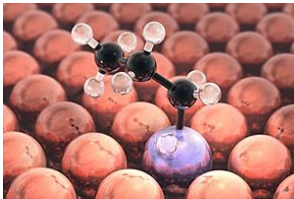
Artistic rendering of the propane dehydrogenation process taking place on the novel single Rhodium atom alloy catalyst, as predicted by theory.
